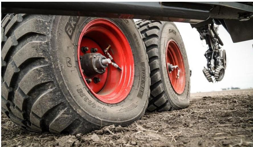
One feature of Load Logic on the Momentum planter is management of tire pressure to ease compaction.
